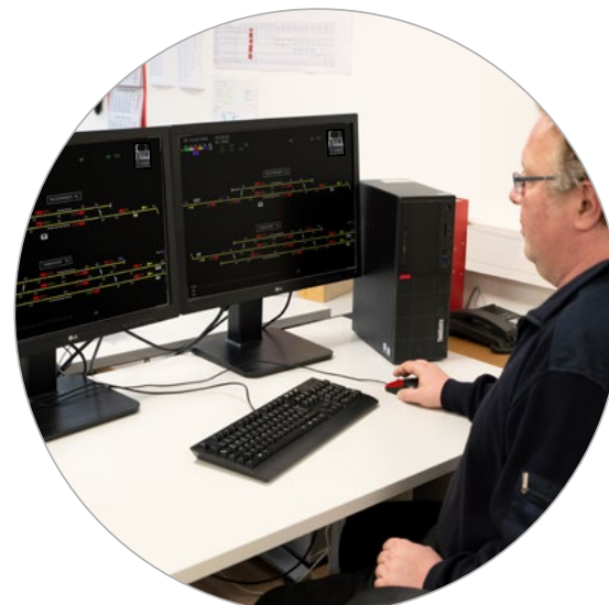
Decentralised operator station with standard PC equipment and DEUTA Trust equipment
