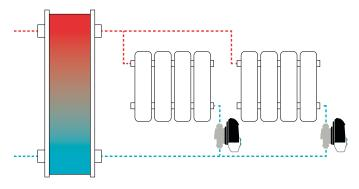
Automatically managing the hydronic balance in new and existing buildings, operating in both ePICV or eDPCV functionalities.
