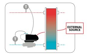
To control delta T, flow, or power in a system, or to maintain a constant third parameter such as indoor temperature, data center cooling bath temperature, and others.
